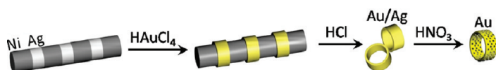
Scheme 1. Scheme illustrating the OWL technique used to fabricate nano-rings. Striped Ag–Ni nanorods (prepared by electrochemical deposition) are used as templates for a galvanic replacement reaction (GRR) followed by selective wet chemical etching of Ni and Ag.
